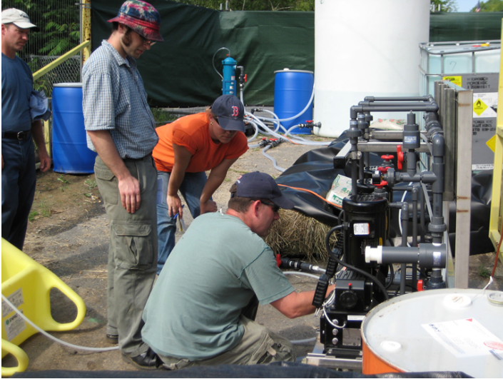
Field application of the VeruTEK surfactant-chemical oxidant mixture. VeruTek's chemical oxidation process will be evaluated for its effectiveness in cleanup of contaminated soil and groundwater at former manufactured gas plant sites.
